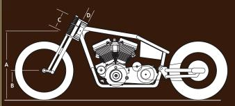
NOTE: Position the frame level and set to final ride height with rear wheel in place to ensure a proper fit
